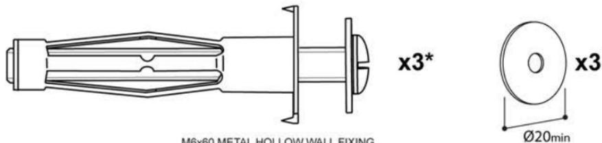
M6x60 METAL HOLLOW WALL FIXING
