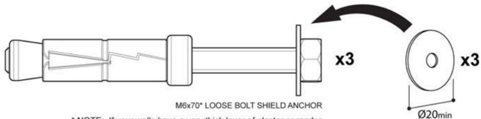
M6x70\* LOOSE BOLT SHIELD ANCHOR
